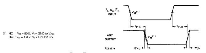
$Fig. 6 \ \ Waveforms \ showing \ the \ input \ (\overline{P}_n, \ C_n, \ \overline{G}_n) \ to \ any \ output \ propagation \ delays \ and \ the \ output \ transition \ times.$
